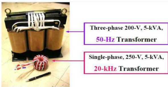
Figure 1: Size comparisons between low-frequency and high-frequency transformers
