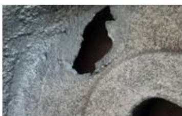
Figure 5: Collapse mold defect
