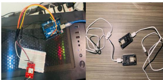
Figure 2: Arduino board, Bread board, Node-mcu, GPS tracker, Jumper wires
