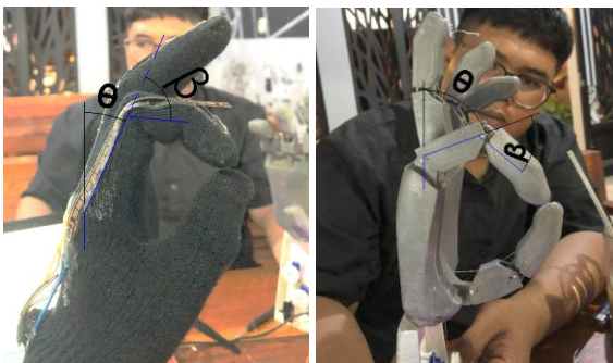
Figure 10: Angle measurement of controller glove and robotic hand
