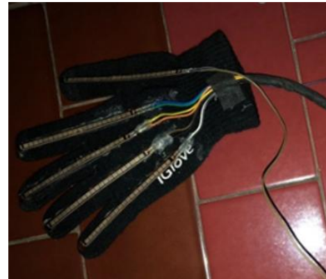
Figure 4: Attachment of Flex sensor on glove
