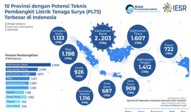
Figure 1: Provinces with the Largest Technical Potential for Solar Power System in Indonesia
