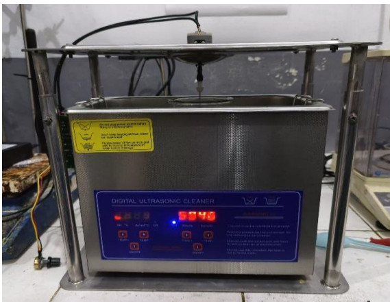
Figure 1: Slurry Mixing with Ultrasonic Cleaner
