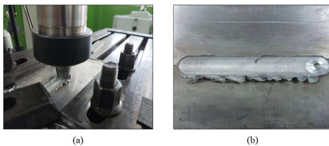
Figure 2: (a) FSW joint process (b) Surface result of FSW joint
